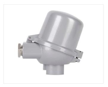
The Type 39 connection head is manufactured from high quality aluminium and is also sometimes known as a BUZ-H connection head. This aluminium housing benefits from two cable entries allowing for easy installation of duplex sensors. In addition this housing can accommodate up to two ceramic terminal blocks or DIN standard transmitters and is weatherproof to IP68. The screwed hinged lid allows for easy access to the sensor and termination.
