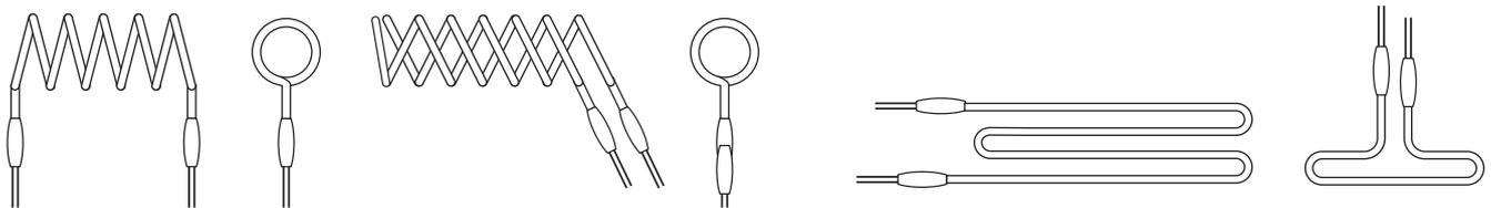
H&B heaters are normally constructed with a cold lead at each end, special heaters can be built with composite elements to supply a variable wattage density or intermediate unheated sections if required see <http://hbsensors.com/products#heaters> for further details.
