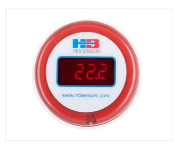
The HBS16001 is a loop powered LED indicator. Powered by a current loop the HBS16001 indicates the process value on a 4 digit LED display. The menu system is easily navigated by the use of three push buttons located on the rear of the display. The HBS16001 can have several linearizations applied or a custom characteristic can be entered.
