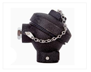
The Type 21 connection head is manufactured from cast iron and is also sometimes known as a KI connection head. This cast iron housing can be fitted with most types of ceramic terminal block or DIN standard transmitter and is weatherproof to IP68. A chain is supplied which connects the lid and body. This connection head is ideal for rugged and difficult environments.
