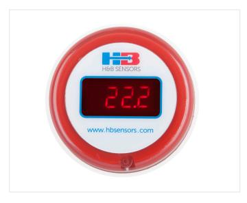
The HBS16001X is an I.S loop powered LED indicator. Powered by a current loop the HBS16001X indicates the process value on a 4 digit LED display. The menu system is easily navigated by the use of three push buttons located on the rear of the display. The HBS16001 can have several linearizations applied or a custom characteristic can be entered.
