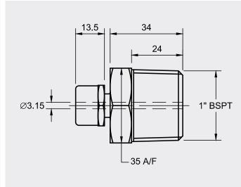
The HBS/4/6600/29 ATEX Exd compression fitting is manufactured from high quality 316 stainless steel. This fitting has a 1" BSPT thread and is suitable for use with 3mm diameter mineral insulated cable.
